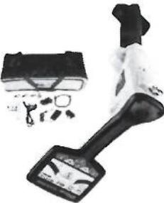
The VLoc3-5000 utility locator is the top devices in the VLoc3 series with the most comprehensive range of features including Bluetooth and GPS, it features both signal direction (SD) and signal select (SIS) the two function is improve the reliable positive line identification in difficult environments and condition.
